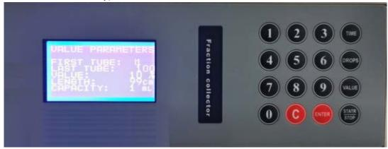
The "first tube" is set to "3" and press "confirm" button; At the end of the "tube" is set to "10" and press "confirm" button; Puts the "VALUE" parameter is set to "50%",
