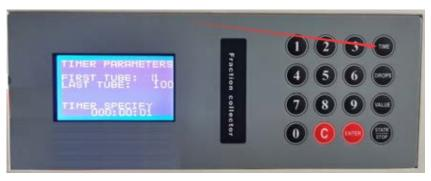
Set the parameter of "FIRST TUBE" to "1" and press "ENTER";
