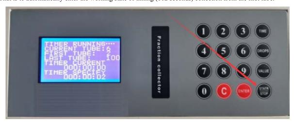
After running to the end of timing collection of tube 100, the instrument will alarm automatically, Press the "START/ STOP" key to clear the alarm
