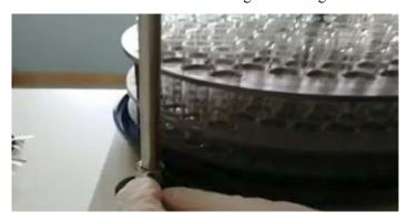
4. Fix the "safety valve" on the upper part of the "vertical bar"
