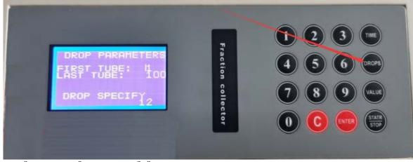
The "first tube" is set to "3" and press "ENTER" button; At the end of the "tube" is set to "10" and press "ENTER" button;
