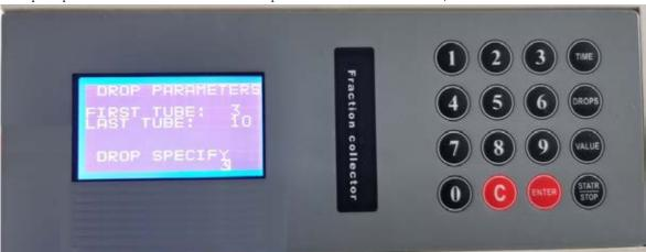
Press the "start/stop" button, Initialization "DROP" into the interface
