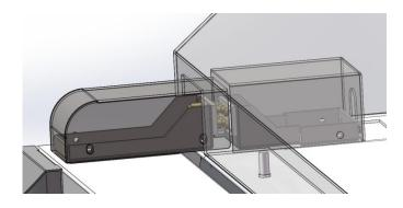
The door contact connector is a structure for supplying power to the test box door. When the door is closed, the contact is turned on, and the heating and illumination on the test box door can work normally. The door contact connector has a working voltage of 24V, which is a safe voltage and does not cause harm to people. If the politeness is dismantled, it is easy to cause the virtual contact of the contact, so that the lighting on the test box door and the heating cannot work normally.
