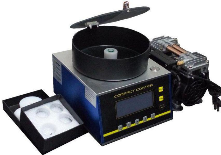
SPC-40 is CE certified compact spin coater with vacuum chucks designed for easy and quick coating via sol-gel for wafers up to 4" diameter. The spinning speed is variable from 100-10000rpm with two programmable segments
